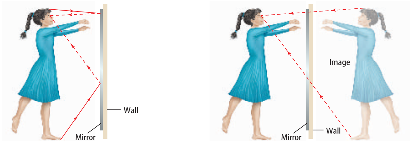
A Light rays that bounce off a person strike the mirror. Some these light rays are reflected into the person's eye. B The light rays that are shown entering the person's eye seem to be coming from a person behind the mirror.
