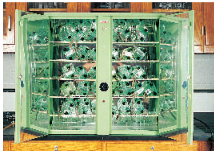
Figure 14 Sterilizing devices, such as this goggle sterilizer, use ultraviolet waves to kill organisms on the equipment.
